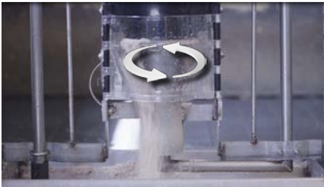
Feed automatically fills when sensor indicates empty trough, according to the adjustable time frame.
