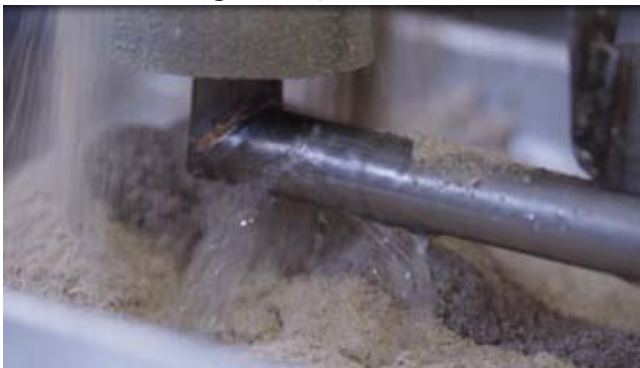
Water and feed are mixed in the bottom of the trough.
